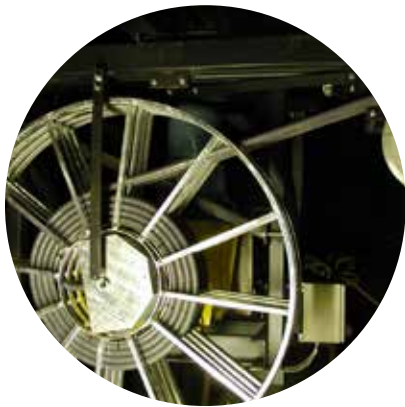
Motorised cable reels
