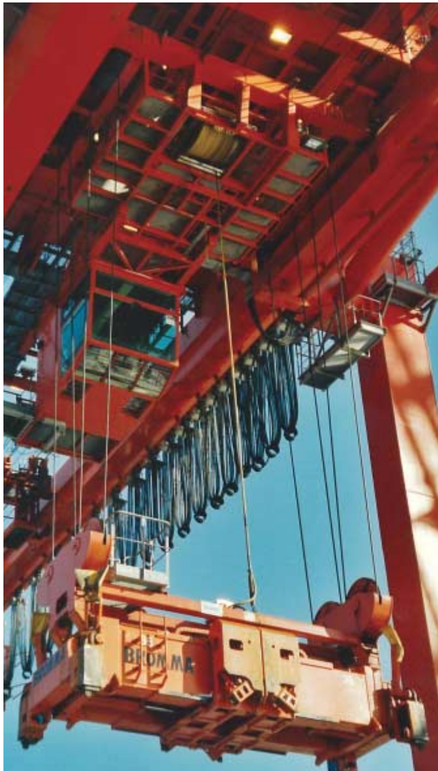
A Cavotec Specimas Spreader Reel in action.
