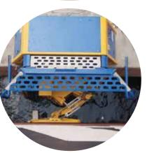
MM200C17 **Product:** Type: Front mounted Capacity:  $12 \times 200 \text{kN} = 240 \text{ tonnes}$ **Moorings:** 3-4 times a week Route: Global **Vessel names: Various** Container vessels up to 392m LOA: Operator: **APM Terminals** Owner: Port of Salalah Since 2009 In operation:
