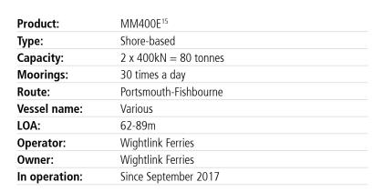
Wightlink began a major upgrade of their terminals at Portsmouth and Fishbourne which also included the purchase of a new-build vessel. With a 89m LOA this vessel required the pier in Portsmouth to be extended to ensure safe mooring. However, due to the layout of the port the extension faced many technical and regulatory hurdles.
