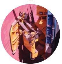
MM200C17 **Product:** Type: Front mounted Capacity:  $14 \times 200 \text{kN} = 280 \text{ tonnes}$ **Moorings:** 1 time every second day Route: Global **Vessel names:** Panamax and mini-Capes LOA: up to LOA 295m Operator: Pilbara Ports Authority, PPA Owner: PPA Since 2010 In operation:
